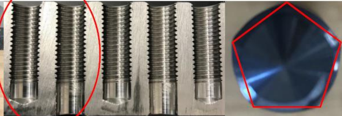
Spike – Thread forms M10 – 3xd – 50 holes
