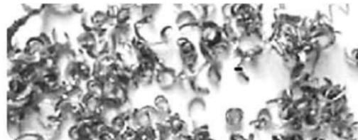
After applying the Chip-breaker
