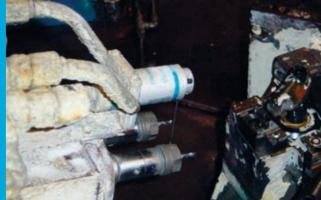
Tool breakage inspection: Bidirectional scanning
