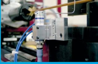
**Workpiece inspection: Checking contours**
