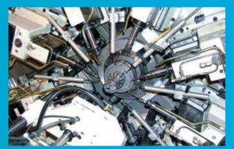
**Workpiece inspection: Checking drill depths**
