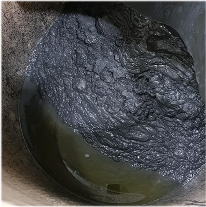
The shape of the sludge discharged from the automatic sludge discharge device
