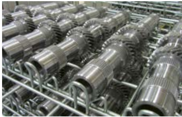
Image 1: Process capable for large production runs - as an example, drive shafts for a manual gearbox machined on a transferline by SNAP-X.
