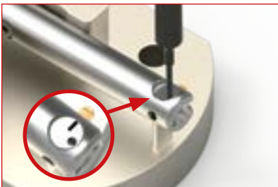
There are a line mark and the black split pin visible (see remark on page 55). Push the split pin through the tool holder by using the smaller diameter of the assembly pin (same direction for disassembly and assembly!).
