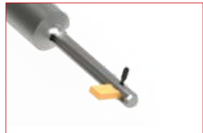
Brake off the assembly aid extensions of the blade and from the roll pin manually.
