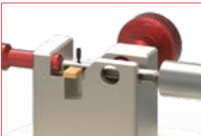
Insert roll pin with its longer and thinner section first.
