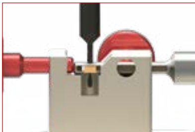
Use assembly pin to push roll pin level with blade. Then unclamp the tool.
